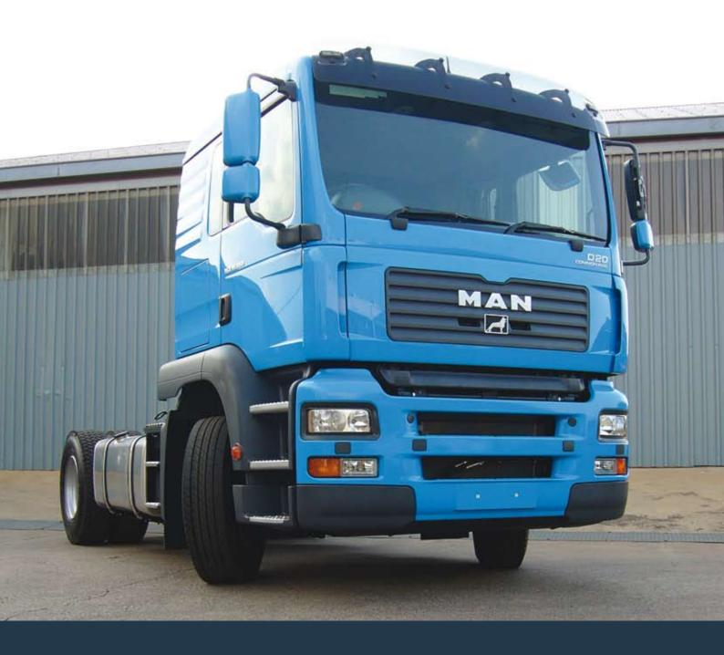
4 x 2 Truck Tractor Single Sleeper Cab D20 Common Rail Engine Air Suspension Hypoid Rear Axle
